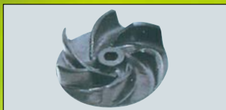
Impeller made of engineering plastic After 200 hours of pump operation Loss of impeller weight:3.3%
